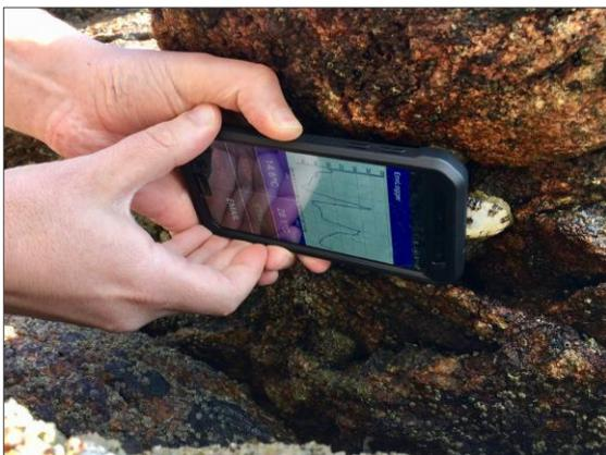
Figure 1 Temperature data being retrieved from an EnvLogger in the field. This particular EnvLogger was previously encapsulated in a limpet shell and attached to the rock surface.
