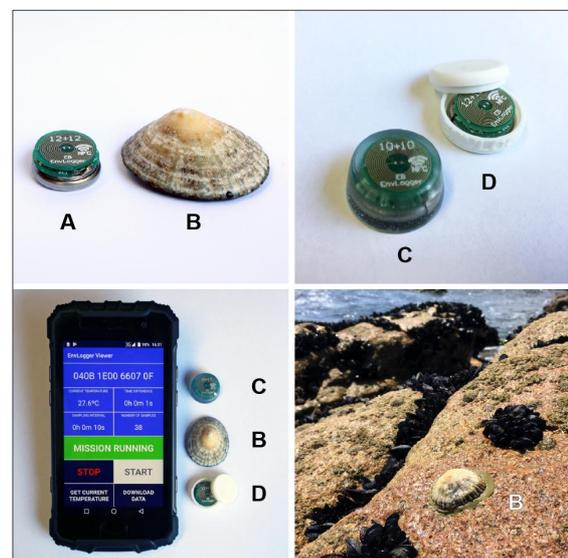
Figure 2. Variety of EnvLogger packages. (A) naked electronics, (B) biomimicking logger (robolimpet), (C) encapsulated in acrylic, (D) enclosed in a 3D printed capsule. B and C can even be safely deployed in the intertidal zone, a hazardous environment for electronics featuring significant wave forces, sharp thermal transitions and salt water corrosion.
