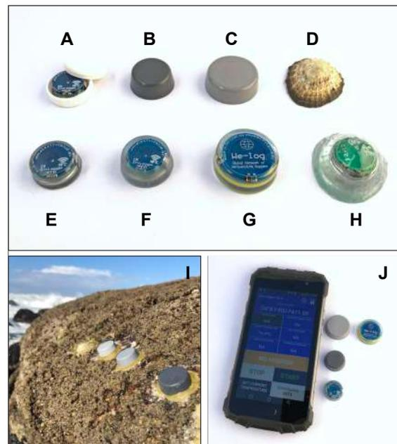
Figure 2. A-H Variety of EnvLogger packages. All but A are highly resistant to dust, water and UV, and can be safely deployed in the intertidal zone, a hazardous environment for electronics featuring significant wave forces, sharp thermal transitions and salt water corrosion (I). A rugged smartphone is all that is needed to communicate with the EnvLoggers in adverse environmental conditions (J).
