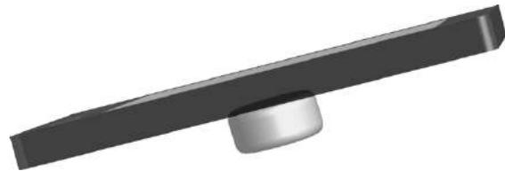
Figure 4. Keeping the smartphone centered with the logger and touching will dramatically improve communications in most models. Note that on some models (e.g., iPhones) the antennae is located on the top of the phone and so the logger should touch that area (near the rear camera).
