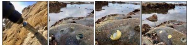
Figure 14. Process of embedding loggers in the rock. From left to right: drilling, clean holes, pressing a logger against Z-Spar<sup>4</sup>, loggers covered in Z-Spar<sup>4</sup>.
